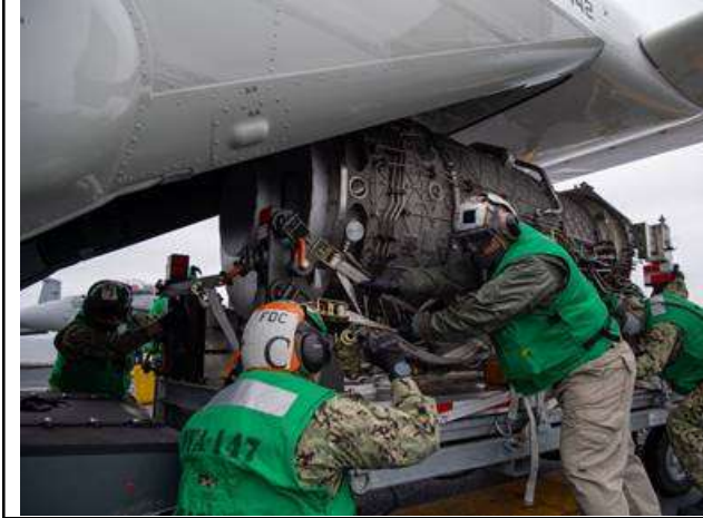
U.S. Navy Conducts First At-Sea Power Module Replenishment
