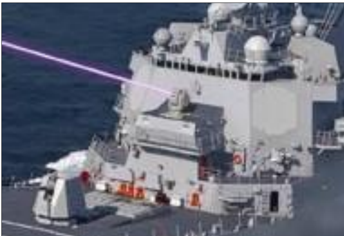
Figure 12. HELIOS System on DDG-51 Destroyer
