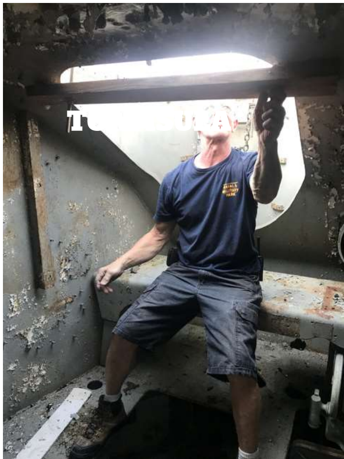
Joe removing the leaking plexiglass cover from inside the cupola of the forward gun director, facing aft.
